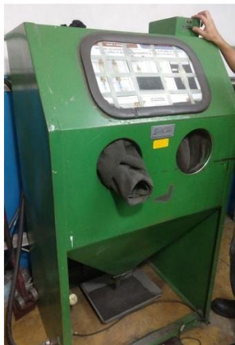
**Figura 3.7.** Máquina de *Sand Blast* Empire Abrasive S-36©
