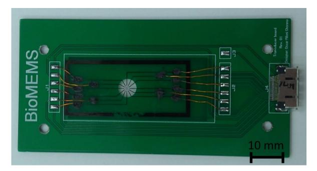
Fig. 28: Photograph of the complete electronics interface board with C-MEMS microelectrodes connected to the PCB.
