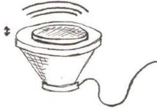
Figure 4.2: As the speaker reproduces the “monochromatic” wave, i.e. the single frequency coming out of the amplifier, the flat plate containing the fluid, fixed to the cone (diaphragm) of the speaker, oscillates.
