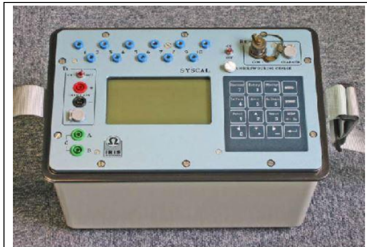
Fig. 18: Resistivímetro Syscal-Pro Switch 48 de Iris Instruments.
