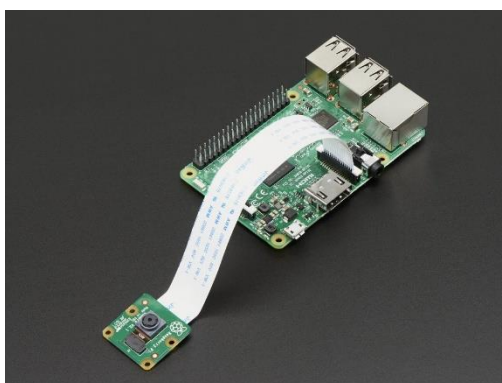
Figura 4.13. Raspberry Pi Camara Board v2 – 8 Megapixeles [4.22].
