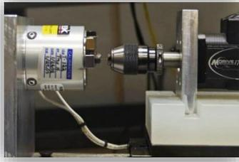
Fig.20 Aparato de prueba de torque. [20] Evolution of nickel-titanium instruments: from past to future.
