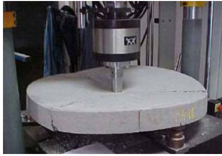
Figura 1.7 Ensayo de panel circular (ASTM C1550)
