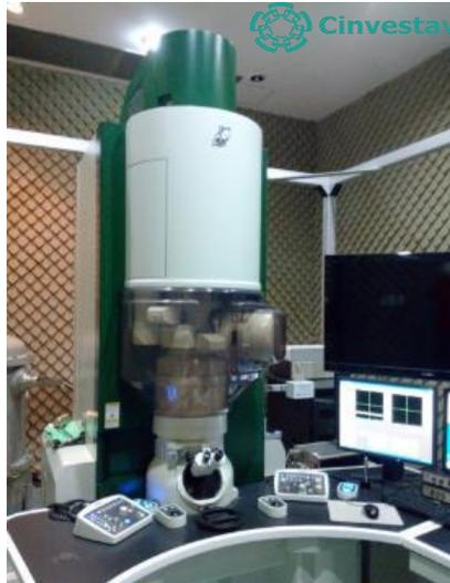
Figura 3.6.7 Microscopio Jeol JEM-ARM200F.
