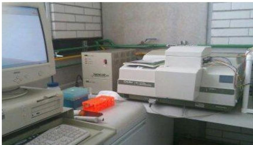
**Fig.19**Espectrofotómetro UV/VIS CARY 1E UV-VIS (VARIAN, INC)
