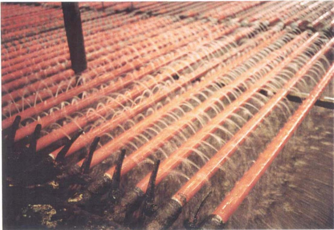
**Figura 3.24. Adición de agua de lavado (Tomada de Mineral producers improve plant performance using column flotation technology)**
