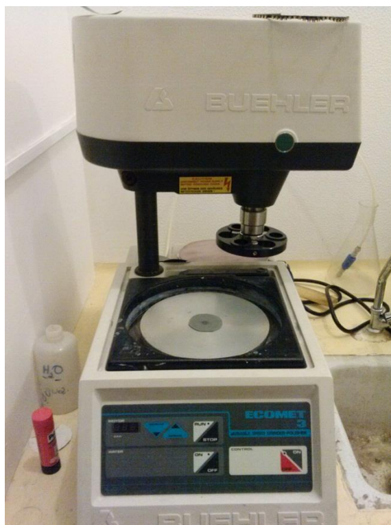
Figura 21. Pulidora ECOMET 3 Variable Speed Grinder- Polisher.
