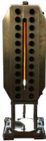
Figura 3.16 Dispositivo de la burbuja ascendente ( www.vinci-technologies.com/products )
