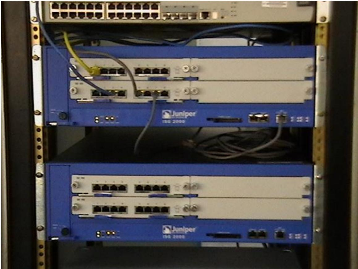
**FIGURA 24. FIREWALL DE LA MARCA JUNIPER MODELO ISG 2000.**
