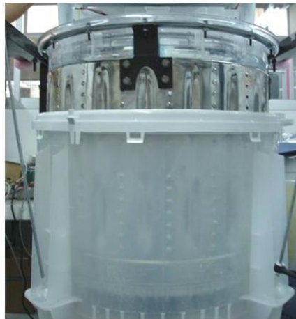
Figure 12. Washing unit for fluid flow visualization and PIV experiments.
