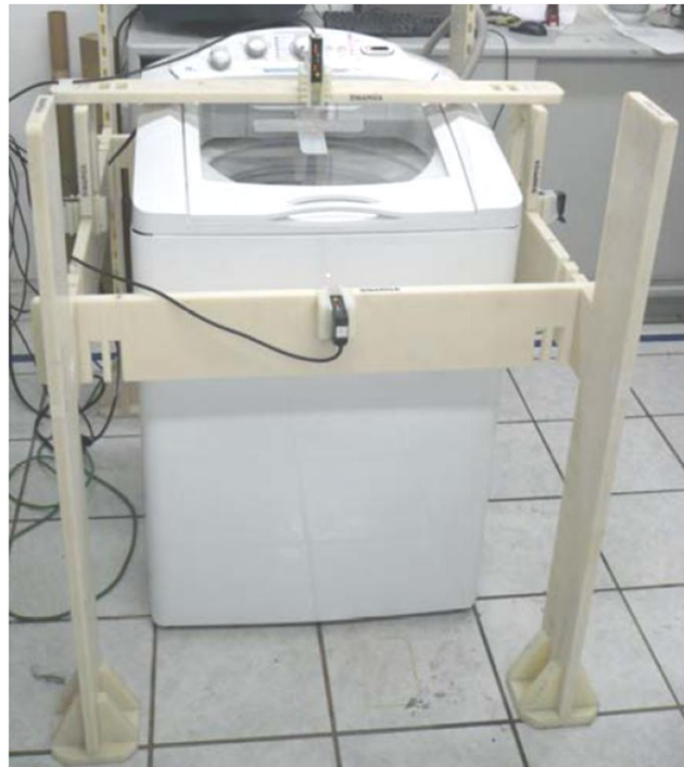
Figure 49. Experimental array for measurements of vibration on the cabinet structure.
