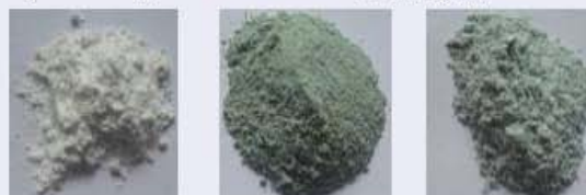
Images of the solid solution of ZnAl_2O_4 , (Zn_{0.9}Ni_{0.1})Al_2O_4 and (Zn_{0.8}Ni_{0.2})Al_2O_4 , respectively, synthesized by the sol-gel method.
