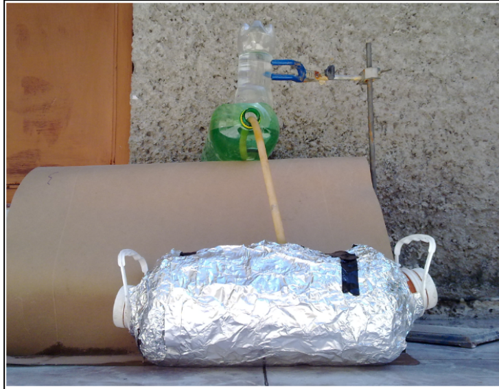
Figura 3.8 Reactor anaerobio experimental a régimen continuo
