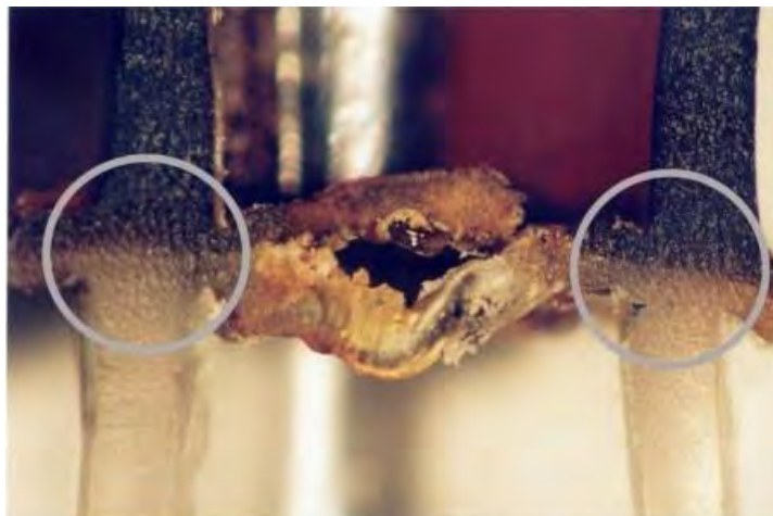
Successfully Sealed Ampoule (The sealing area has a mixed color)
