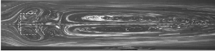
Figure 3.12: Experimental observations in GalnSn alloy for Re = 100 and Ha = 50 . The visualization of flow was obtained using 4% HCl solution covering the metal surface (Kolesnikov et al. 2008).
