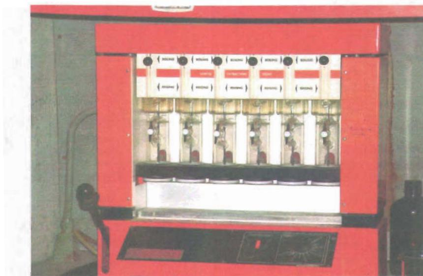
Figura 2. Extractor Soxtec System HT6
