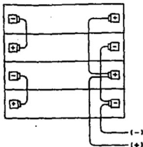
FIG. 4.20 CONEXION DE DOS GRUPOS EN PARALELO,
