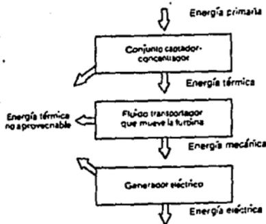
FIG. 4.7 ESQUEMA DEL PROCESO TERMODINAMICO SOLAR
