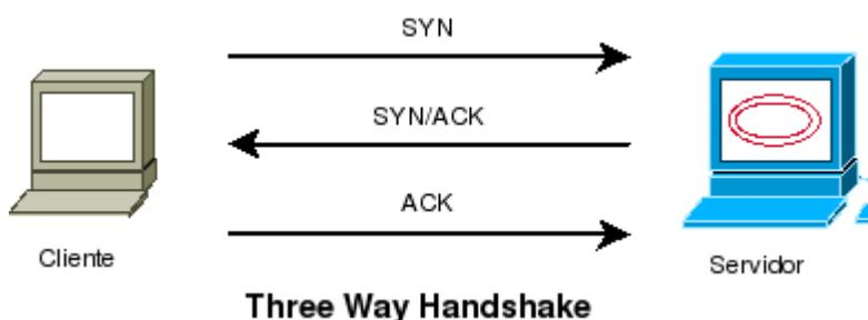
**Figura 3.7.** Three Way Handshake
