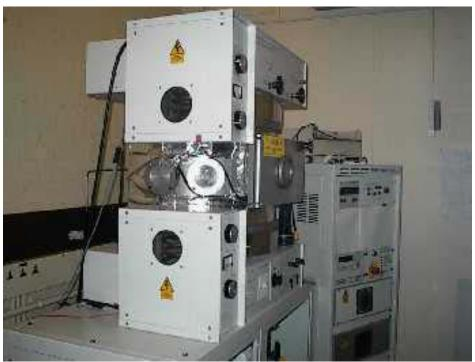
Fig. AI.5 NORDIKO NM2000 RF magnetron sputter deposition system
