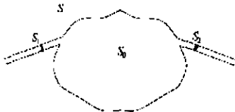
FIG. 3. A ballistic cavity with reflection symmetry described by the matrix S_0 , connected to two waveguides by means of two barriers described by S_1, S_2 . The barriers give rise to direct processes and, if they are different, the LR symmetry of the full system is broken (external mixing).
